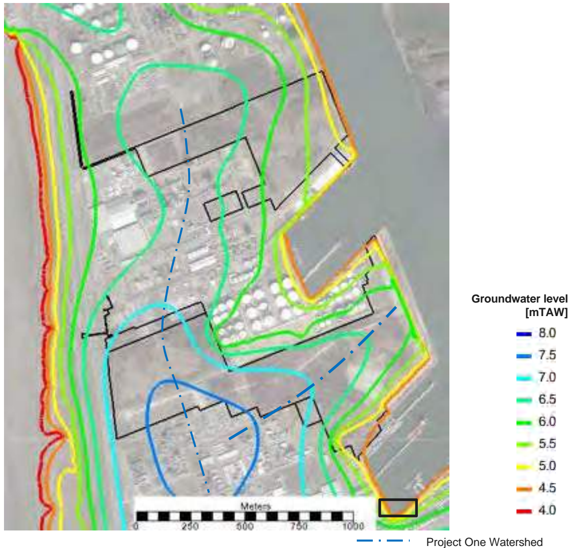
Figure 9-3: Groundwater level (m TAW) in the current situation in the phreatic aquifer, including the permitted construction of the quay wall (dotted lines: watersheds)
