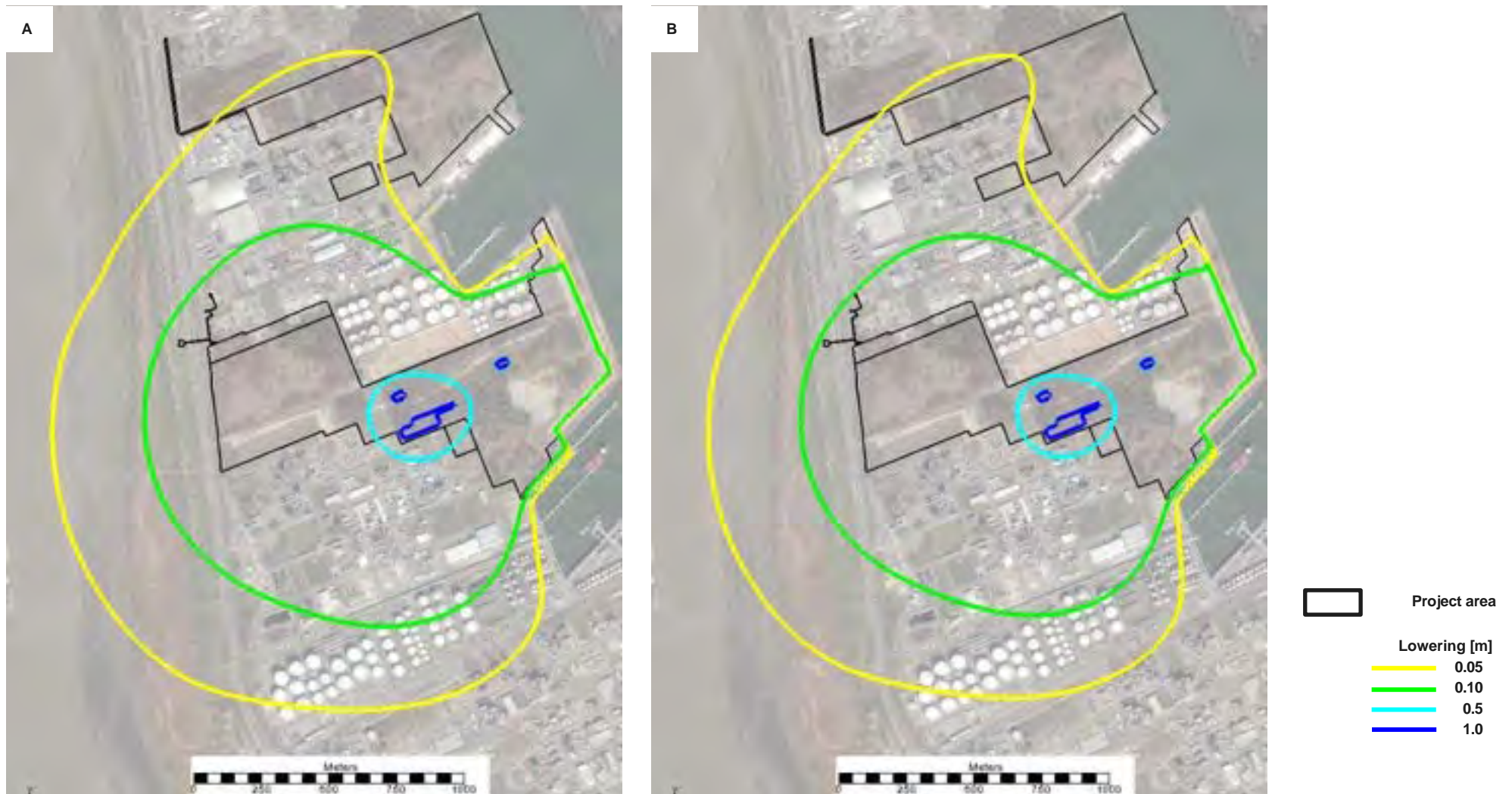
Figure 9-18: maximum calculated groundwater reduction (m) in the second aquifer for a) maximum scenario (drainage without measures) (left), b) sheet piling scenario: drainage with preventive measures, i.e. installing sheet piling around the construction zone
