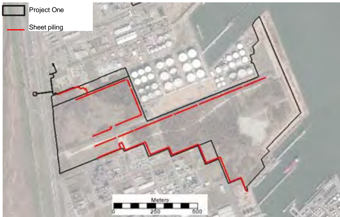
Figure 9-10: Location of the sheet piling during the construction phase
